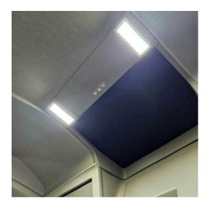
Step One: Remove Existing Light panels place 2 x holes as per below to allow the wiring from the LED Panels
