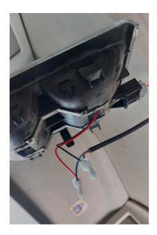
4. Connect the Red lights cable with the cable that we extended between the led plates (driver's side)
