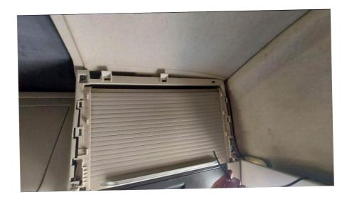
5. Repeat the same process on the other side (co-driver's side) and extend a second double core cable by removing the cover of the cupboard
