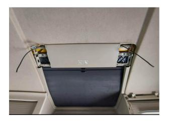
3. Pass a double core cable between the led plates (watch picture)
